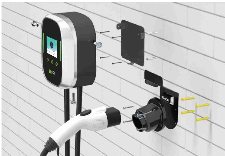
Figure 4-3 General Installation Drawing
